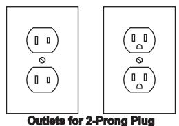
1. Tools marked "Double Insulated" do not require grounding. They have a special double insulation system which satisfies OSHA requirements and complies with the applicable standards of Underwriters Laboratories, Inc., the Canadian Standard Association, and the National Electrical Code. (See Outlets for 2-Prong Plug.)  Double insulated tools may be used in either of the 120 volt outlets shown in the preceding illustration. (See Outlets for 2-Prong Plug.)
